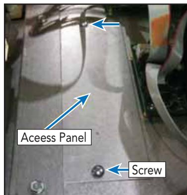
The image to the left shows the access panel. Access to the lower latch will still require removal of the oven for service.
