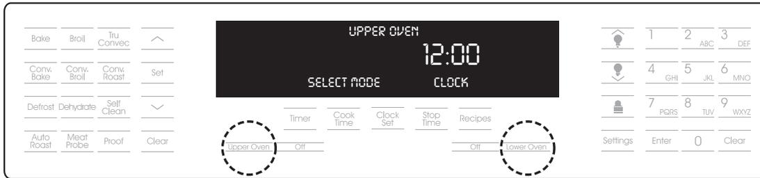
2. Depress the "SETTINGS" button on the control panel. You will see the word SETTINGS in the upper left corner of the screen and the BRIGHTNESS parameter.
