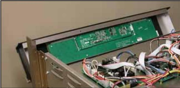
5. Remove screws securing touch board.
