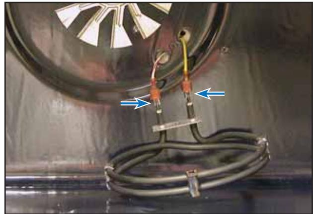
5. Repair or replace convection element as necessary.
